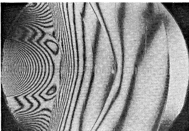
Fig. 5.11 Density contours computed by the time-split upwind TVD scheme (4.34a,c,f) compared with interferograms at approximately the same time instants.
