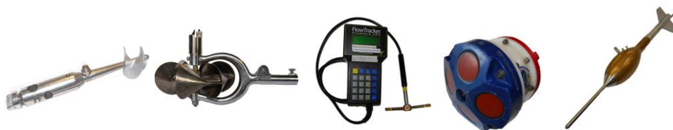
Figure 1 – Examples of velocity current meters. From left to right; Rotating-element propeller, Rotating-element cup, ADV, ADCP, POEM. Photographer: A Willsman, NIWA.
