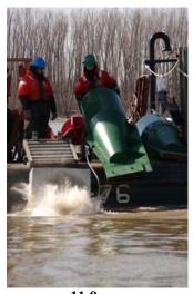
11-9 Deploying Sinker with Dump Board
