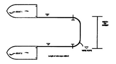
Figure 14-2 Two Boat Wire Sweeping Diagram
