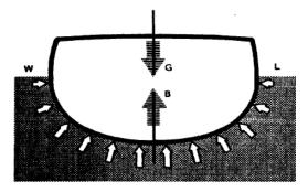
Figure 7-1 Centers of Buoyancy and Gravity
