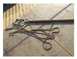
Figure 4-30 Line Reeving Device
