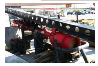
Figure 12-3 Hammer and Lead in Cradle
