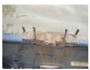
Figure 11-5 Wire Rope Fairlead Device
