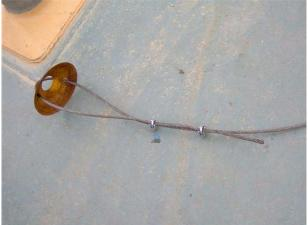
Figure 11-7 Jet Cone Mooring on Deck
