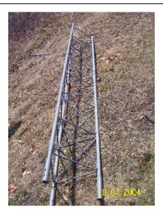
Figure 11-11 10ft Rohn Tower Section
