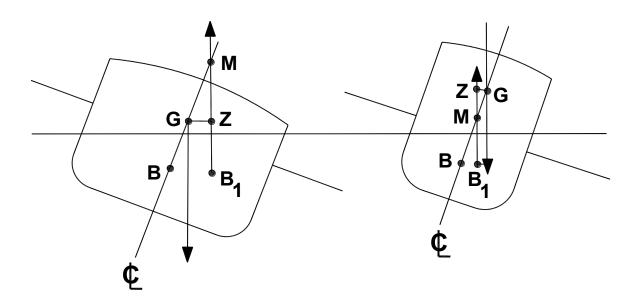
Figure 7-3a Vessel in stable condition
