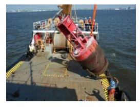
Figure 9-3 Centering the Buoy on the Deck
