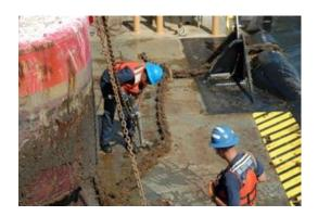
Figure 9-5 Griping Down a Buoy
