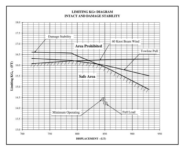
Figure 7-4 Limiting KGv Diagram
