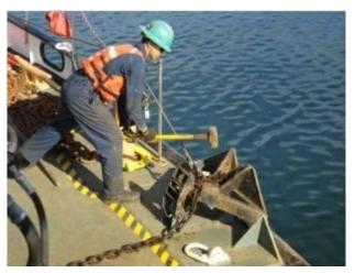
Figure 10-2 Setting the Chain into the Stopper
