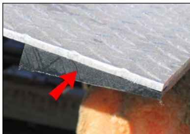
6 inch gangplank wearstrip wedge
