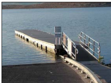
single-rail steel beam guided boarding float
