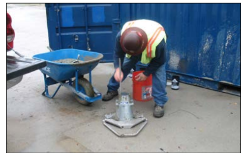
performing concrete slump test
