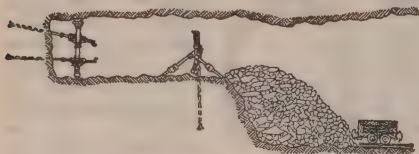
Fig. 82. Top Heading and Bench Method
