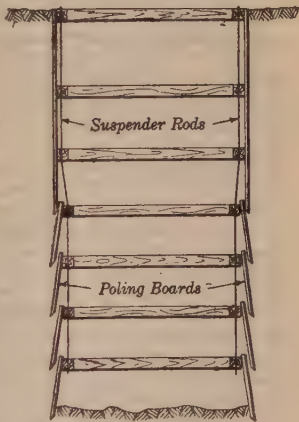
Fig. 25. Poling Board Method
