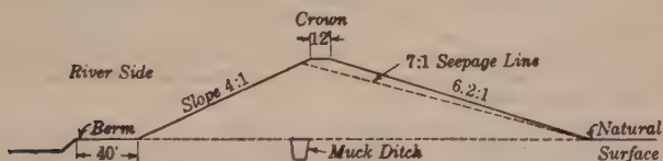
Fig. 40b. Proposed New Levee Section
