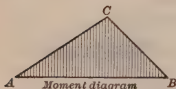
Fig. 33. Beam Supported at Ends, Concentrated Load at Any Point in Span.
